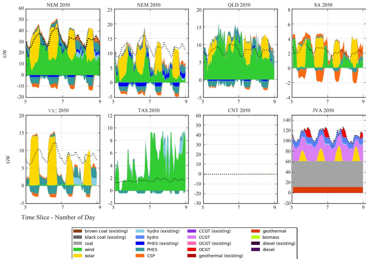
Fig. 5 Time series snapshot of the hourly dispatch (GW) for each of the states/regions in scenarios one and two. Figures show 4 days out of the total of 28 days used in the optimisation. The dot line shows the state energy demand
