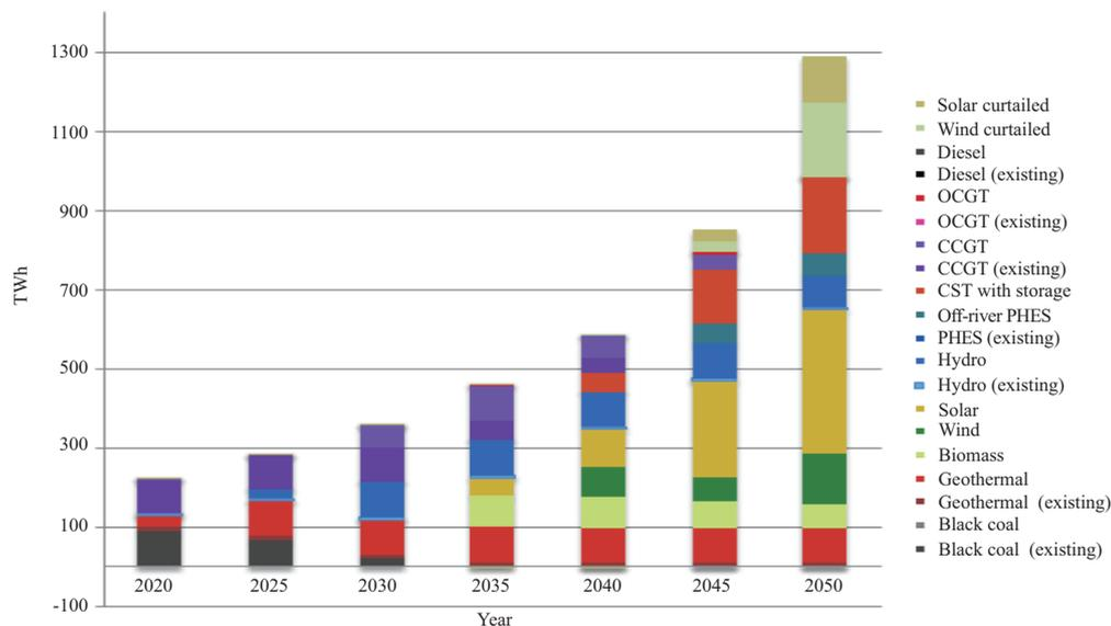
**Fig. 6 Scenario 3, energy generation for Java-Bali with the 100% emission abatement with all demand met with domestic capacity. Note the high levels of curtailment of wind and solar PV**
