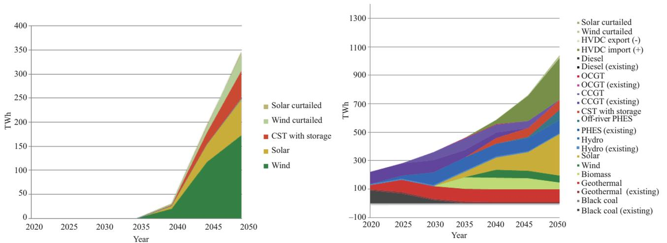
Fig. 9 Energy generation (and imports) for CNT (left) and Java-Bali for scenario 4 (HVDC switched on)
